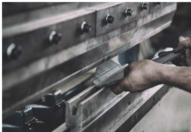
7 CNC bending the steel plates for the supports.
