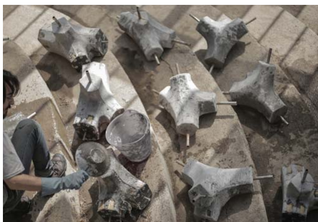
6 Treating the demolded nodes with water to reduce the cracking rate.
