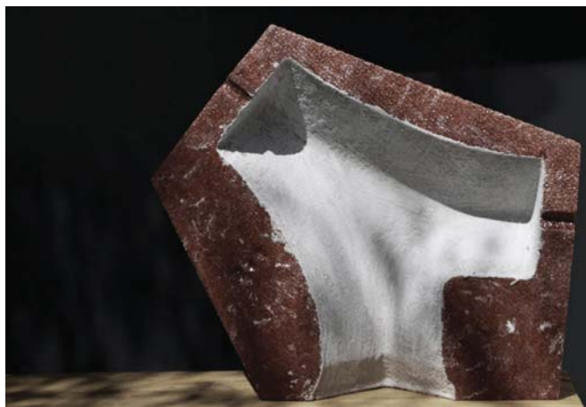
5 Coating foam molds and preparing them for concrete casting.
