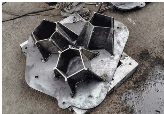
8 A completed support including bent steel plates welded to the base surface.
