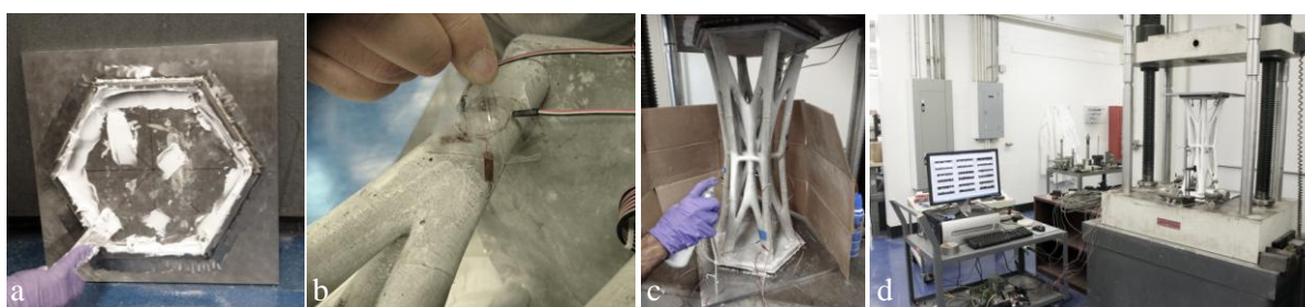
Figure 3: Test setup; (a) cap, (b) strain gage installation, (c) spraying the specimen, (d) test setup
