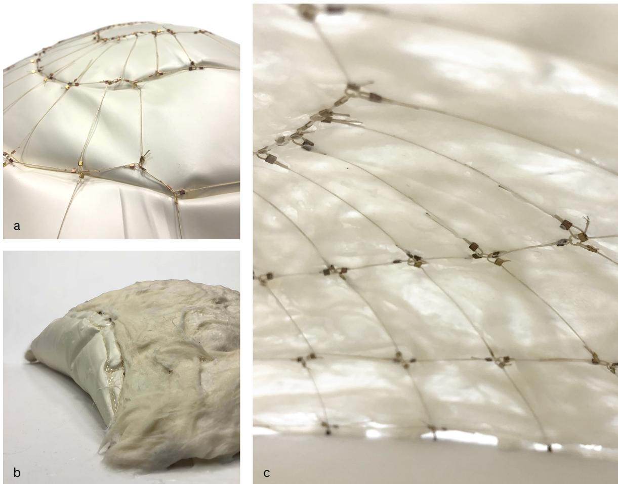
Figure 8: Physical Model Construction: (a) pneumatic formwork constrained by wireframe network, (b) wax-fiber composite placed on pneumatic formwork, (c) wireframe network embedded within wax-fiber composite.
