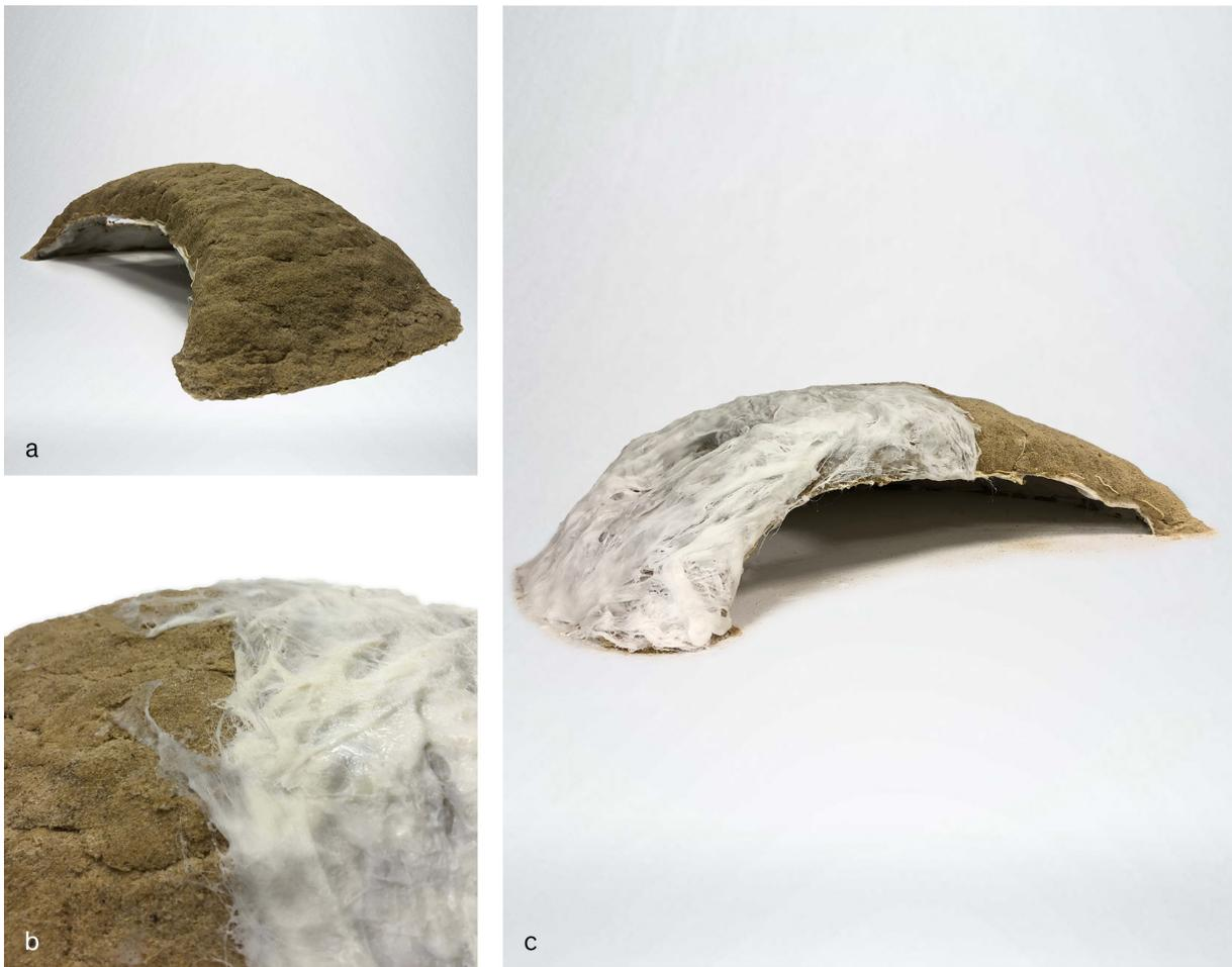
Figure 9: Physical Model Construction: (a) terrene mixture solidified into crescent dome structure, (b, c) wax-fiber composite placed on exterior of terrene mixture.
