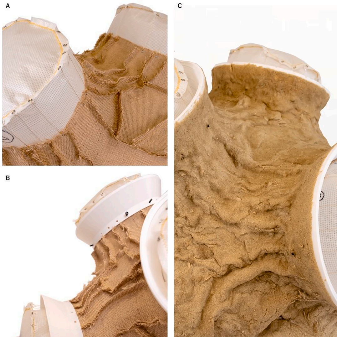
Fig. 8. Global Fabrication Steps: A) application of burlap sleeve to pneumatic formwork, B) anchoring of PLA frames to burlap, C) ChitoSand administered to burlap exterior.
