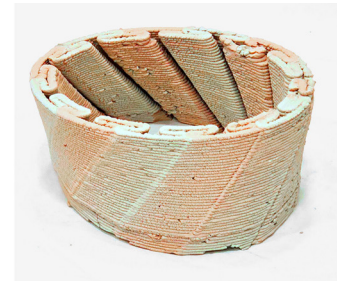
6 Material composition control through the SNMM extruder system.
