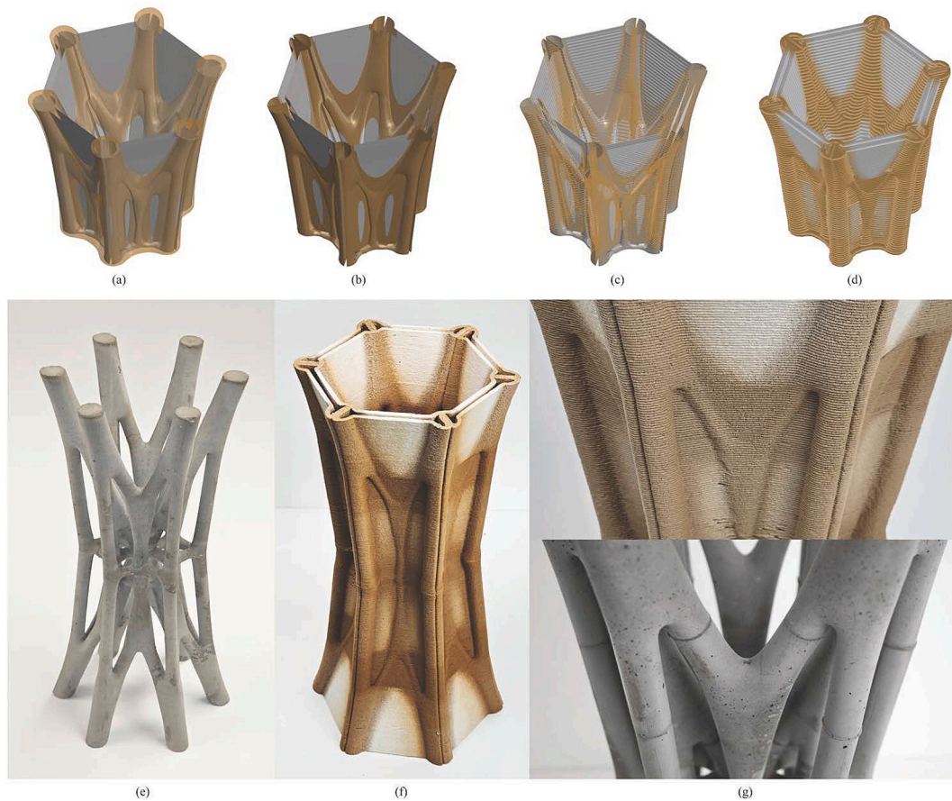
Fig. 12. SNMF printing of a funicular polyhedral column: (a) the base geometry (gray) and the intersector (brown); (b) divided surfaces; (c) multimaterial toolpath curves generated based on the surface division; (d) the toolpath visualization (layer height exaggerated for display); (e) the base geometry cast using concrete with a height of 250 mm in [73]; (f) the final print with a height of 250 mm; and (g) the comparison details of the two artifacts.
