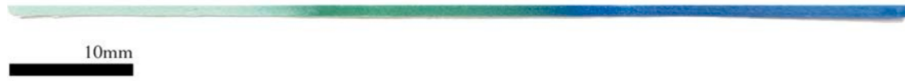
Fig. 3. The sample print of a continuous line with three segments of different colors.
