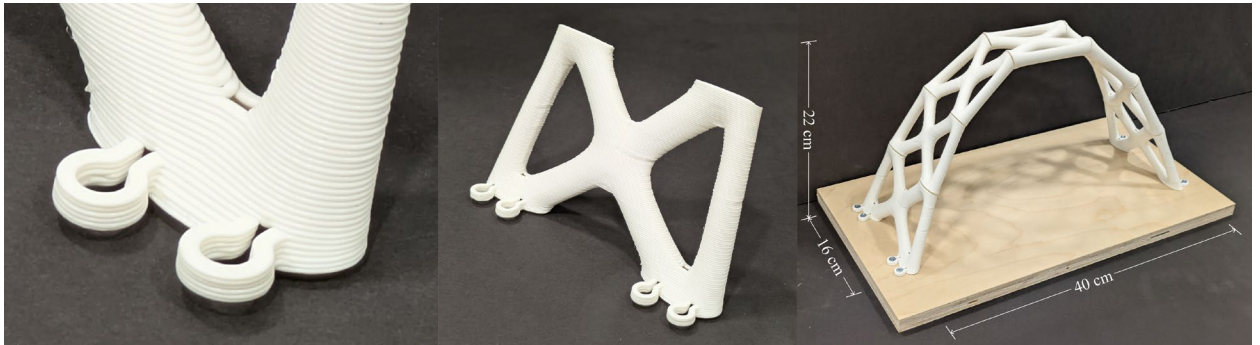
Figure 16: Scaled fabrication model of the discrete arch with 7 components. Each component takes around 1 h 30 mins to print.
