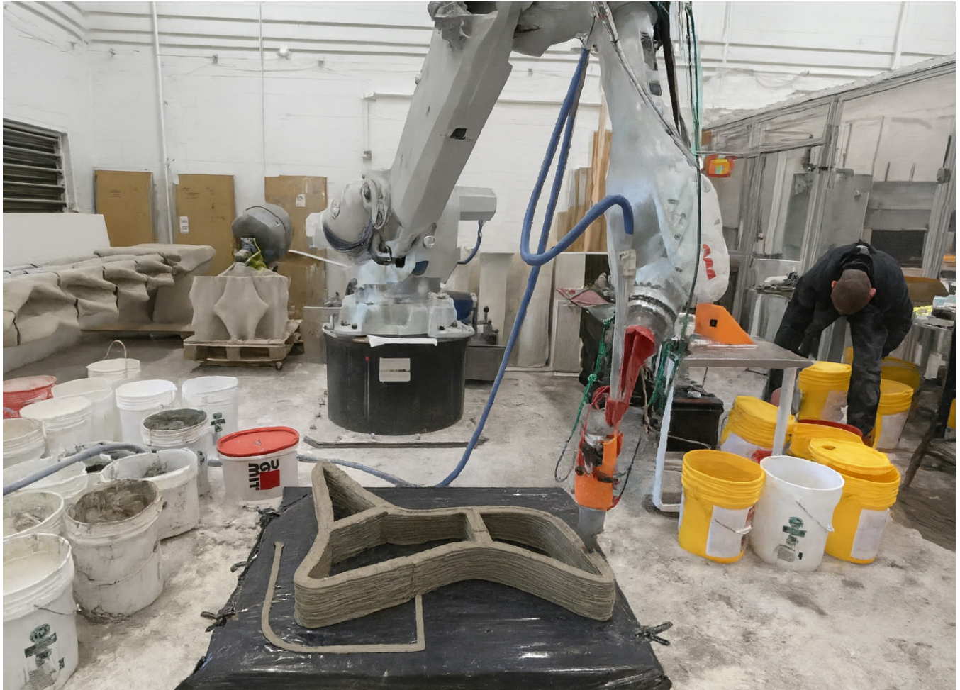
8 Robotic concrete 3D printing process of a geometric toolpath designed as a continuous loop to enhance printability.
