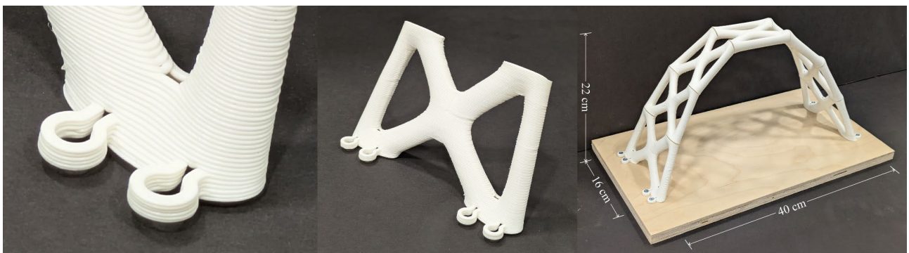
Figure 20: Scaled fabrication model of the discrete arch with 7 components. Each component takes around 1h 30 mins to print.
