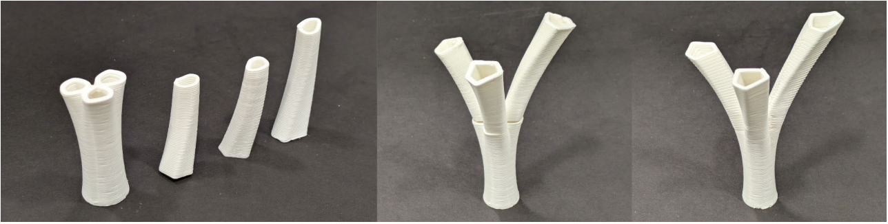
Figure 23: Scaled fabrication models of the branching node in two configurations.
